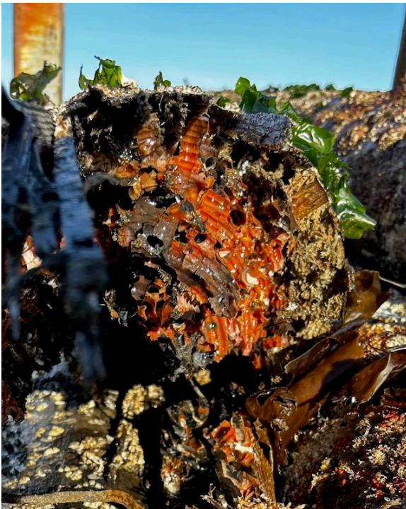
Wormholes in a pile that broke off while pulling.
